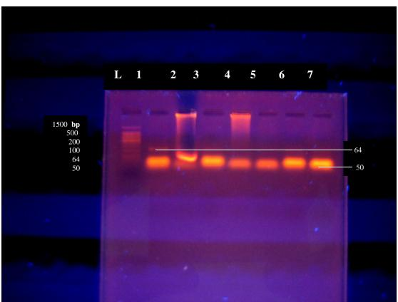
Fig .2. Hsp 92II restriction fragments of COMT alleles separated by agarose gel electrophoresis. L, Ladder. Lanes 3,6,7 show a homozygous low activity allele (Met/Met), Lanes 4,5 show a homozygous high activity allele (Val/Val), and Lanes 1,2 the heterozygous pattern
