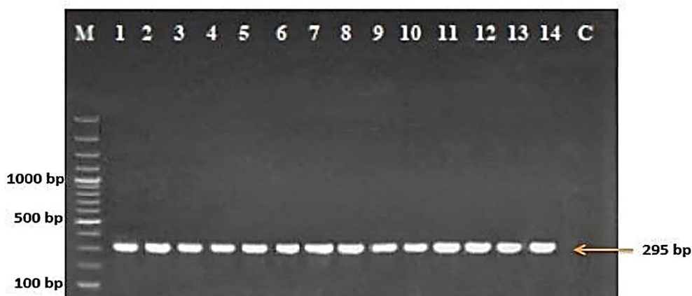
Figure 5: Gene amplified by electrophoresis. Visualization was accomplished using 1% agarose electrophoresis and ethidium bromide staining at 75 V for 1 hour. 100 bps DNA ladder is the marker for Lane M. Positive samples for the lasI gene (295bp) are shown in lanes 1-14. Lane N: Negative control.
